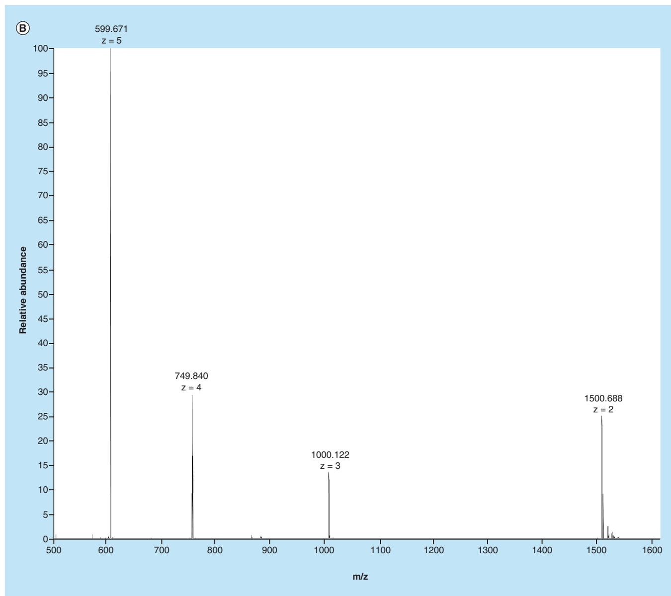
**Figure 3.** LC-high-resolution mass spectrometry analysis of REVERSIR-A in monkey plasma (cont.). Sample was collected 2 h after a 3.0 mg/kg sc. dose of REVERSIR-A. (A) Total ion chromatogram. (B) Electrospray ionization mass spectrum of Rev-N1-N9 metabolite. (C) Isotopic envelopes for the charge state of five for the Rev-N1-N9 metabolite. (D) Deconvoluted mass spectrum of the Rev-N1-N9 metabolite.
