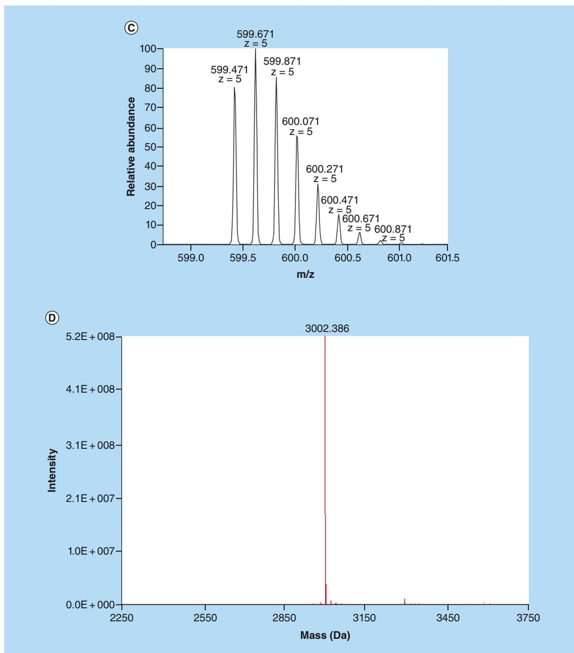
**Figure 3.** LC-high-resolution mass spectrometry analysis of REVERSIR-A in monkey plasma (cont.). Sample was collected 2 h after a 3.0 mg/kg sc. dose of REVERSIR-A. (A) Total ion chromatogram. (B) Electrospray ionization mass spectrum of Rev-N1-N9 metabolite. (C) Isotopic envelopes for the charge state of five for the Rev-N1-N9 metabolite. (D) Deconvoluted mass spectrum of the Rev-N1-N9 metabolite.
