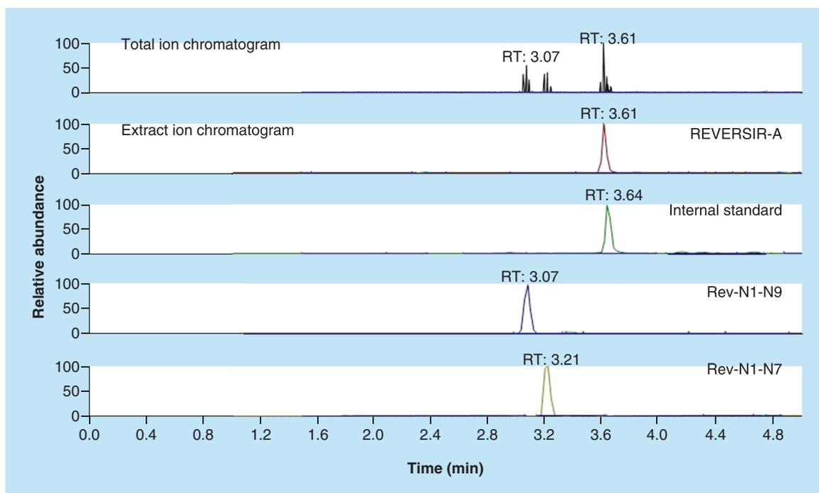
**Figure 2.** LC-high-resolution mass spectrometry chromatograms for spiked REVERSIR-A and metabolites in rat liver homogenate. The blank rat liver homogenate was spiked with 3500 ng/ml of REVERSIR-A and Rev-N1-N9 and Rev-N1-N7 metabolites.
