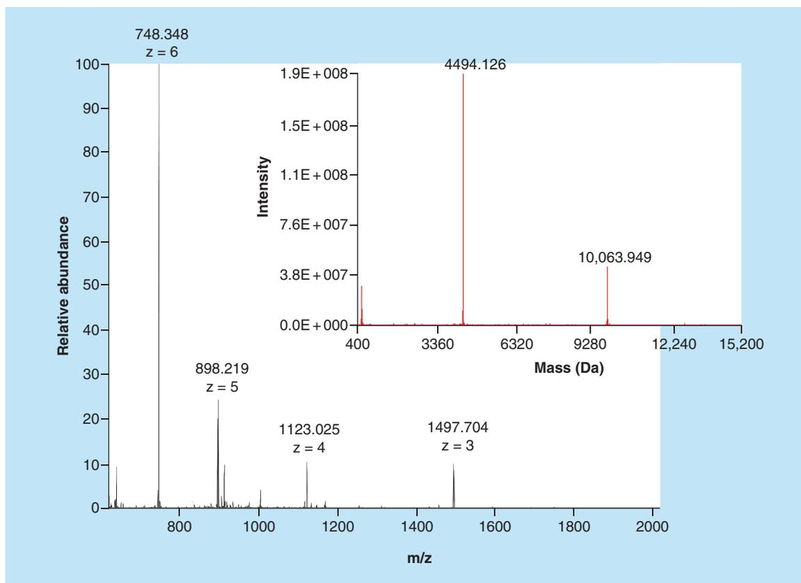
**Figure 5.** Electrospray ionization mass spectrum of the peak at 16.68 min in a monkey liver sample. The insert displays the deconvoluted mass spectrum of the peak. The liver sample is as described in Figure 4.
